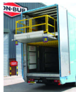
Typical two tier tail lift complete with safety hand rails and three-way ramps.
