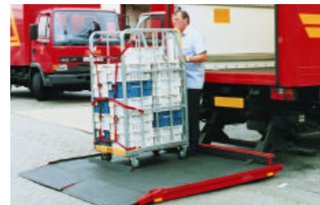
Above: A column tail lift with three-way ramps/rolling load restraints. Left: A large flat platform cantilever tail lift with edge restraints and trolley stops.
