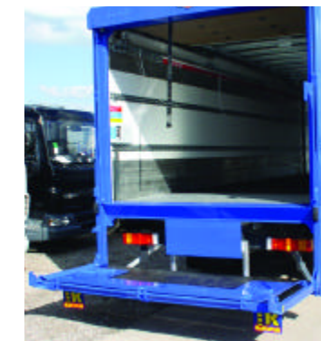
Above: A column tail lift with three-way ramps/rolling load restraints. Left: A large flat platform cantilever tail lift with edge restraints and trolley stops.
